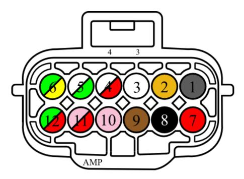
Connector harness fits directly to the mating alarm ECU harness, above diagram shows connector view only (looking at front Yellow connector support panel) all wiring locations are at rear of this connector.
